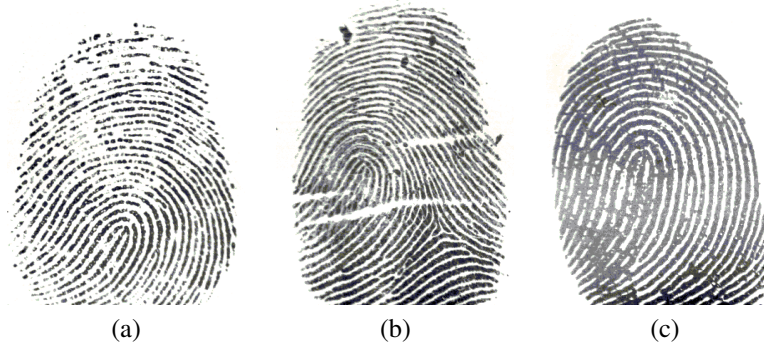
Figure 1. Fingerprint samples taken from the CrossMatch database of the Fingerprint Liveness Detection Competition 2009 [13]: a) live; b) silicone spoof and c) gelatin spoof.
