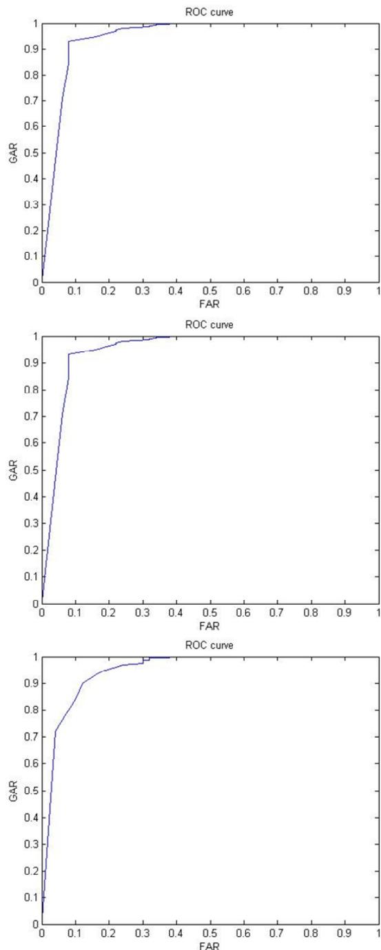
Fig 6. ROC curves of test data and for multi-distance conjunctival vasculature matching, using one eye. Top: 1 ft distance, 6.5% EER; middle: 5 ft distance, 7.4% EER; and bottom: 9 ft distance 11% EER.
