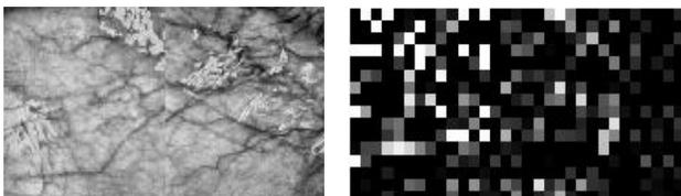
Fig. 3. Left: an input image obtained by mosaicking the scleral regions to the left and right of the iris. Right: the resulting CDF 9/7 wavelet feature matrix ( $16 \times 32 = 512$  features).
