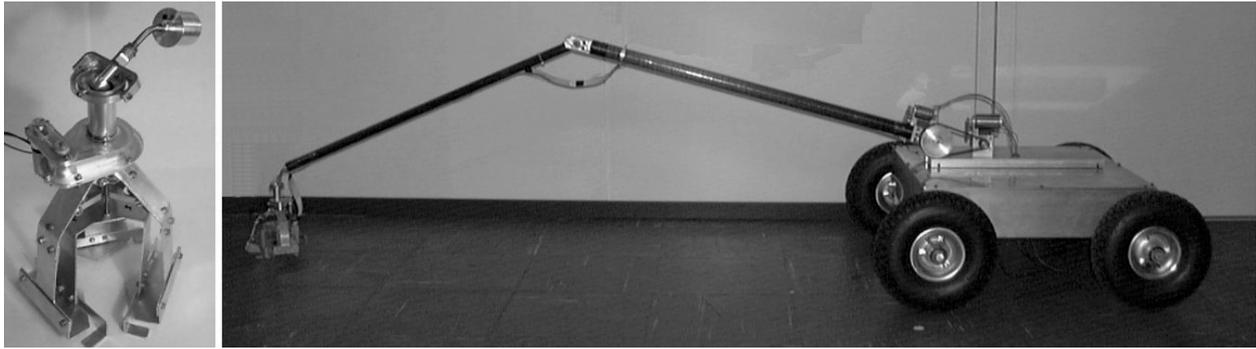
Fig. 1. Prototype three fingered gripper with wiper blades and compliance gimbal (left), and the arm and gripper system mounted on a turn table (right)
