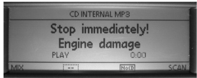
Fig. 7. Exemplary low-tech attack on multimedia system interfaces.
