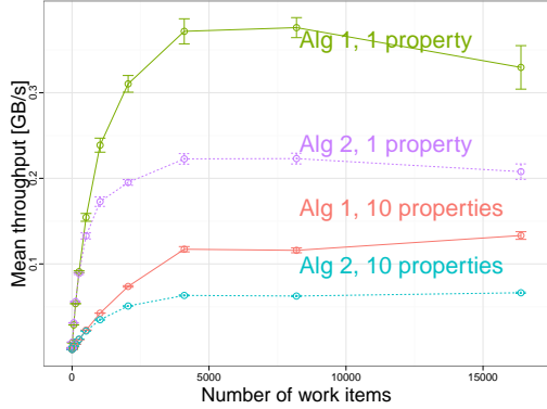
Figure 8. Throughput analysis - throughput vs. the number of work items.
