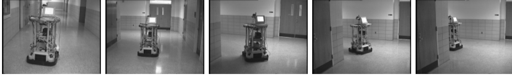
Figure 16: The mobile robot Rome running SHOSLIF navigates autonomously at a walking speed, along hallways, turning at corners and passing through a hallway door. The real-time, on-line, incremental learning and the real-time performance is accomplished by an on-board Sun SPARC-1 workstation and a SunVideo image digitizer, without any other special-purpose image processing hardware. No active sensors, such as sonars or infrared sensors were used.
