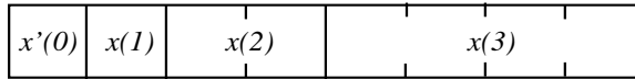
Figure 5: The state representation at t = 3 for 1-D signal with 2:1 uniform resampling in space, from sensory inputs x(0), x(1), x(2), \dots . For this illustration, \mathcal{S} is an 8-dimensional space. x'(0) is the average of x(0) and the initial zeros in the state vector.
