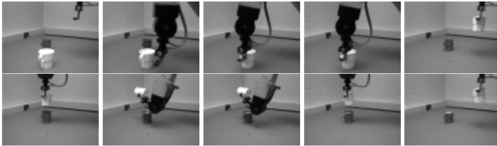
Figure 9: A demonstration of various actions learned: approaching the handle of cup A, picking the cup up, moving to top of cup B, pouring, and putting on table.
