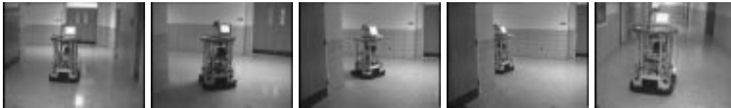
Figure 8: The mobile robot running SHOSLIF navigates autonomously at a walking speed, along hallways, turning at corners and passing through a hallway door. The real-time, on-line, incremental learning and the real-time performance is accomplished by an on-board Sun SPARC-1 workstation and a SunVideo image digitizer, without any other special-purpose image processing hardware.
