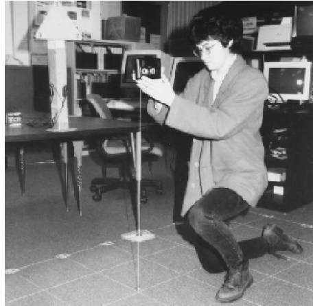
Figure 12: Training the system. The compact sensor array is shown at the upper left corner of the figure. A tape recorder plays the sentence at a predefined height right above a floor grid point. A weight is used to guarantee vertical displacement between the grid point and the tape recorder.
