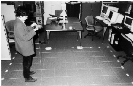
Figure 11: The experimental setup. The compact sensor array is shown at the top of the pole standing on the edge of the center table. The intersection points on the grid on the floor mark the control points in the work space.
