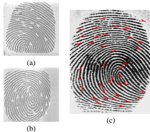
**Fig. 1.** Fingerprint images acquired using the solid state Veridicom sensor (a,b) and the optical Digital Biometrics sensor (c). The detected minutiae points have been marked in the fingerprint images (17 in (a), 21 in (b), 39 in (c)).
