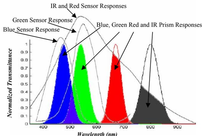
Figure 2. The normalized transmittance of the band-pass prisms and sensor spectral response of the acquisition device. Filled portions of the graph indicate the actual combined response of the sensors and prisms.
