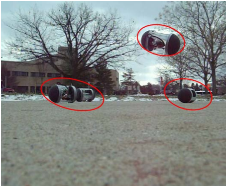
Fig. 2. Hopping sensors we designed in jumping action
