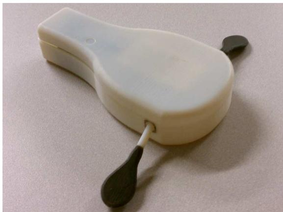
**Figure 2: A hand-designed prototype of the robot produced with multiple materials. The feet are composed of both soft and rigid materials. This initial prototype had a completely rigid arm which resulted in a small contact area between the foot and surface during movement producing slippage of the feet on the surface.**
