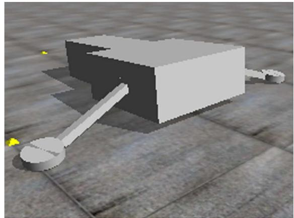
**Figure 1: Initial morphology of the virtual robot. Body is fixed to accommodate motor and batteries in a real robot. The flexible joint is located between the arm and cylindrical foot. Different flexibilities allow for a variable contact area of the foot and ground.**
