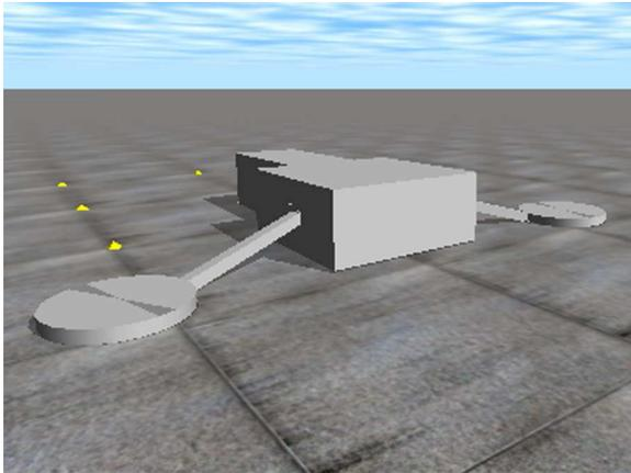
**Figure 5: Evolved morphology demonstrating flexibility of the passive joint as it makes contact with the surface. In this morphology, the foot comes into full contact with the ground with the aid of a flexible joint at the arm-foot junction. The foot size also increased giving the morphology a greater contact area with the surface.**
