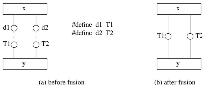
Figure 5.1 Component Fusion via Call Renaming
