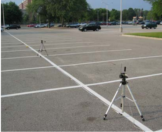
Figure 5: Outdoor Data was collected in an open flat parking lot with two tripods to raise the sensor nodes.
