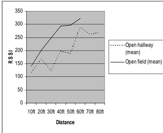
Figure 3: Signal strength behaves differently in indoor and outdoor environments. Signal strength does not correlate with distance in the open indoor hallway.
