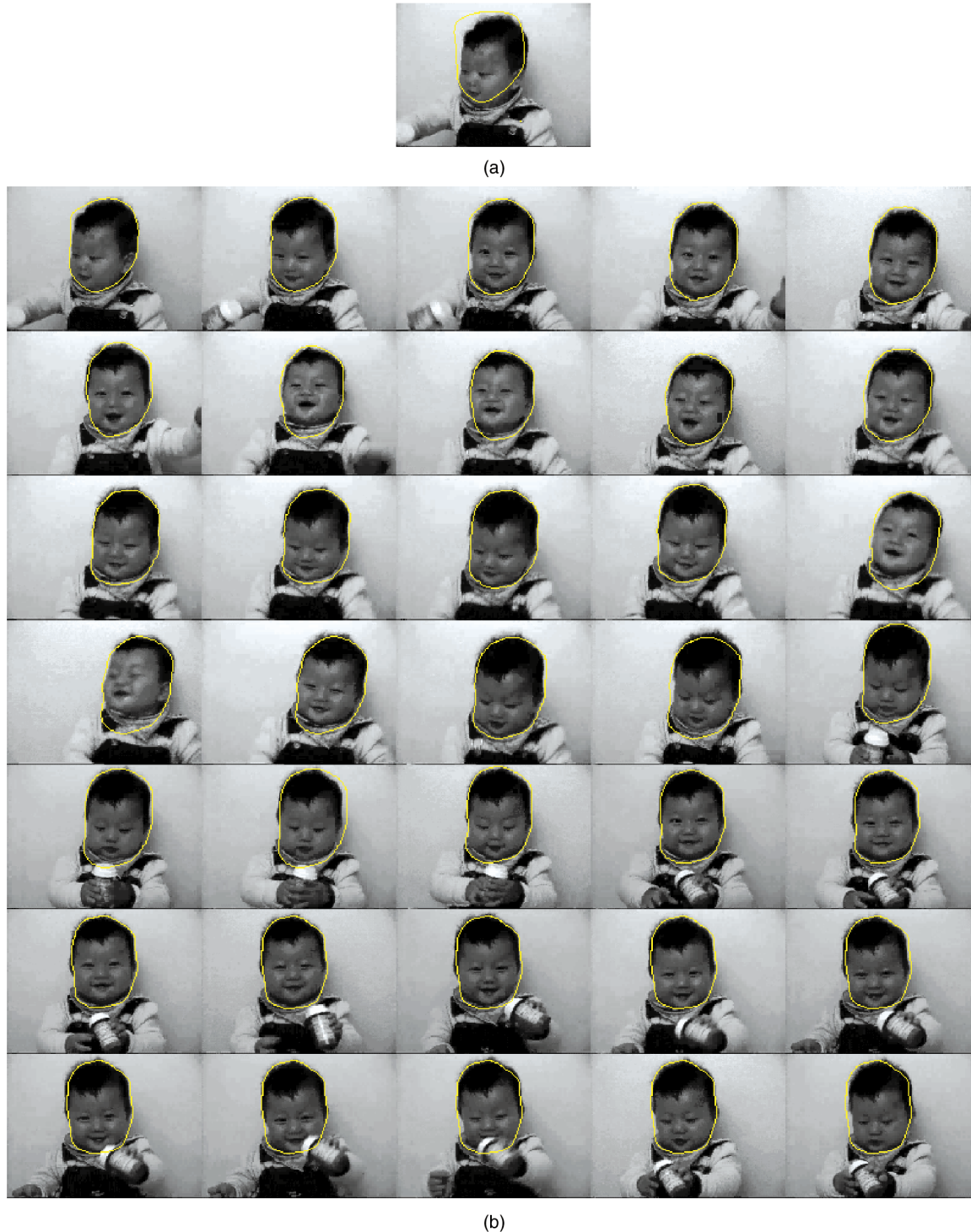
Fig. 3. Tracking a human face in an image sequence (each frame size is 120 \times 160 ). (a) Template initialization in the first frame and (b) tracking results for the sequence.
